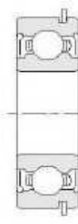
Snap ring or both snap ring With dust cover on both sides (2ZNR)
